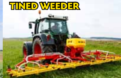
Tined weeder Available working widths: 1,5-15 m
